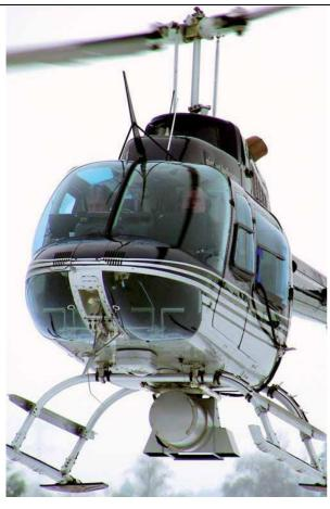
The ALMA G2 (Airborne Laser Methane Assessment Generation 2) is the solution for effective and economic pipeline and storage network monitoring and inspection.
