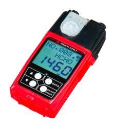
The portable formaldehyde gas detector model FP-31 is a precision gas analyser which measures gases in the ppm range using photoelectric photometry method with chlorimetric detection tabs. This device is a highly sensitive portable instrument with an easy to read LCD display. The unit is capable of detecting very low levels of formaldehyde, in order to confirm if an area contains safe breathing levels.
