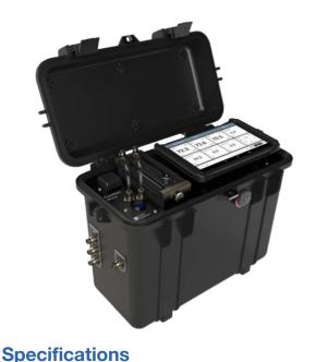
The Fumigation Mate is a four gas, 3 channel fumigant monitoring instrument with a powerful, user friendly integrated fumigation job management system. Providing secure measurement, collection, processing and reporting of all required fumigation data.
